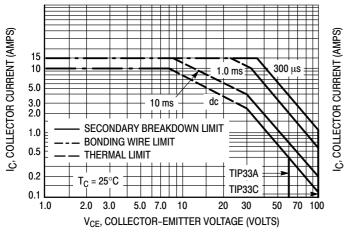
Figure 2. Maximum Rated Forward Bias Safe Operating Area
