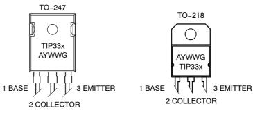
TIP33x = Device Code A = Assembly Location
