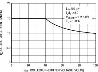
Figure 3. Maximum Rated Forward Bias Safe Operating Area
