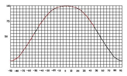
Flux Characteristics @ 350mA, T<sub>j</sub>=25°C
