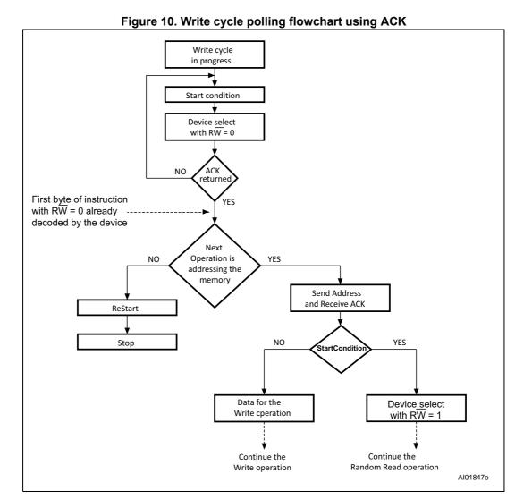
The seven most significant bits of the Device Select code of a Random Read (bottom right box in the figure) must be identical to the seven most significant bits of the Device Select code of the Write (polling instruction in the figure).
