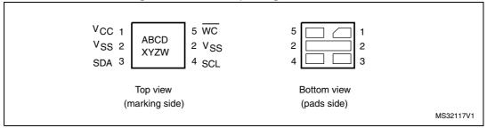
Inputs E2, E1, E0 are not connected, therefore read as (000). Please refer to Section 2.3 for further explanations.
