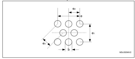
Table 22. M24128-DFCS6TP/K, WLCSP 8-bump wafer-level chip scale package\_related mechanical data
