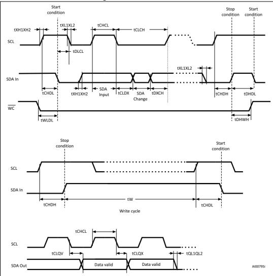
Figure 15. AC waveforms
