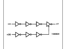
Fig.5 Logic diagram (one buffer).
