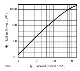
Figure 6. Radiant Power vs. Forward Current
