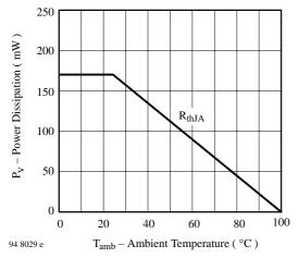
Figure 1. Power Dissipation vs. Ambient Temperature
