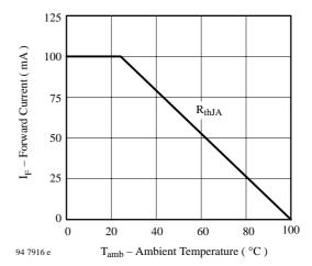
Figure 2. Forward Current vs. Ambient Temperature
