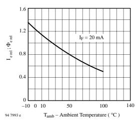
Figure 7. Rel. Radiant Intensity\Power vs. Ambient Temperature
