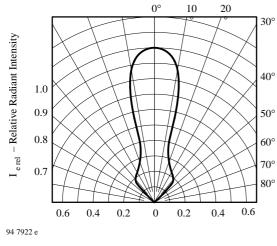
Figure 9. Relative Radiant Intensity vs. Angular Displacement
