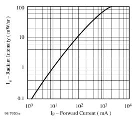
Figure 5. Radiant Intensity vs. Forward Current
