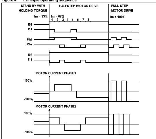
Figure 4. Principle operating sequence
