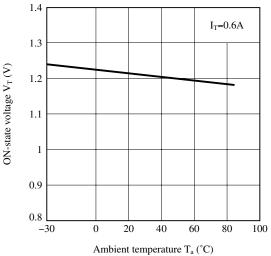
Fig.7 Zero-cross Voltage vs. Ambient Temperature
