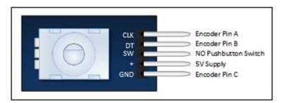
The module is designed so that a low is output when the switches are closed and a high when the switches are open.
