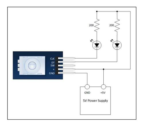
VERY SLOWLY rotate then encoder shaft both clockwise and counterclockwise. Notice which LEDs change state first with rotation.
