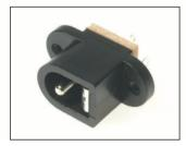
DC-13 panel mounting pin / ring type with switch. Rated 12V / 5A. DC-13A with 2.1mm dia. pin. DC-13B with 2.5mm dia. pin. DC-13A (FC681492) DC-13B (FC681493)
