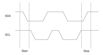
**Stop Condition:** A low-to-high transition of SDA with SCL high is a Stop condition. After a read sequence, the Stop condition will place the EEPROM in a standby power mode (see Figure 6-2).
