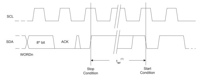
Note: 1. The write cycle time t<sub>WR</sub> is the time from a valid Stop condition of a write sequence to the end of the internal clear/write cycle.
