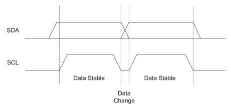
**Start Condition**: A high-to-low transition of SDA with SCL high is a Start condition that must precede any other command (see Figure 6-2).
